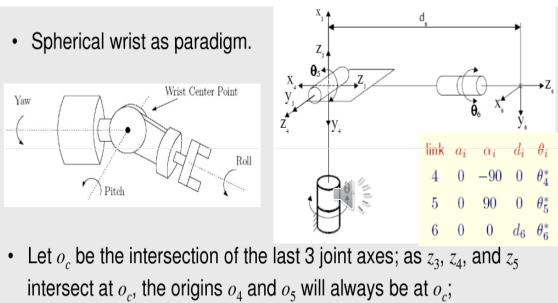
the motion of joints 4, 5 and 6 will not change the position of  $o_c$ ; only motions of joints 1, 2 and 3 can influence position of  $o_c$ .
