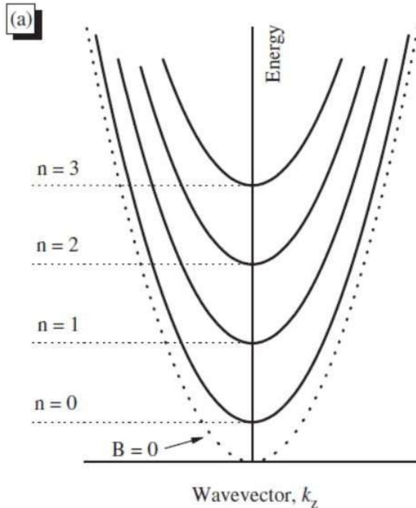
Electron energy bands for a 3D solid vs the  $z$ -direction wave vector for different Landau levels ( $n = 0, 1, 2 \dots$ )
