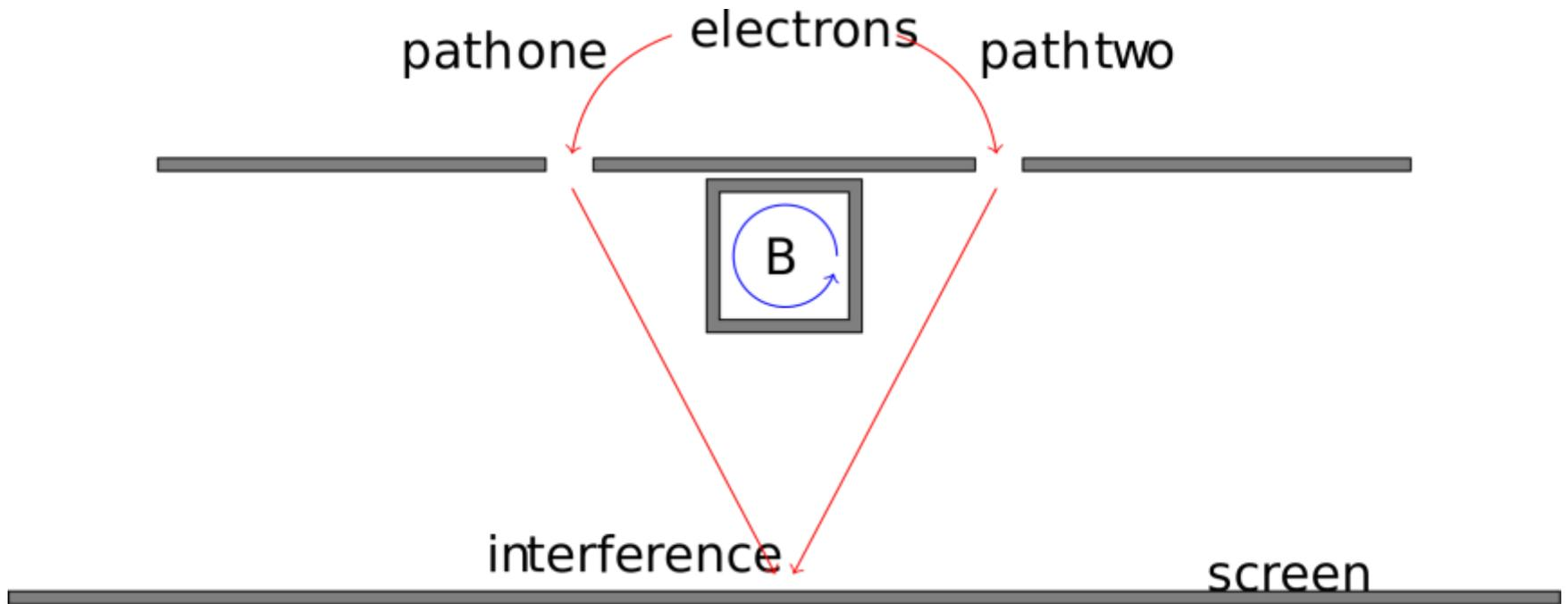
Schematic of double-slit experiment in which the Aharonov–Bohm effect can be observed: electrons pass through two slits, interfering at an observation screen, with the interference pattern shifted when a magnetic field  $\mathbf{B}$  is turned on in the cylindrical solenoid
