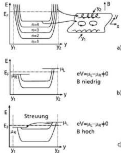
a) the resulting Landau-levels after applying a magnetic field, b) highest Landau-level far away from Fermi-energy - no scattering, c) highest Landau-level near the Fermi-energy - scattering possible [3]
