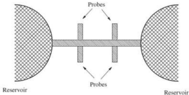
Diagram of a typical nanostructure used to make quantum Hall effect measurements
