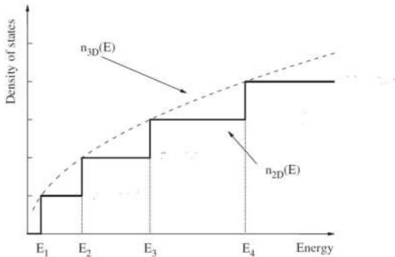
Density of states function for a 2D electron system, as a function of energy.
