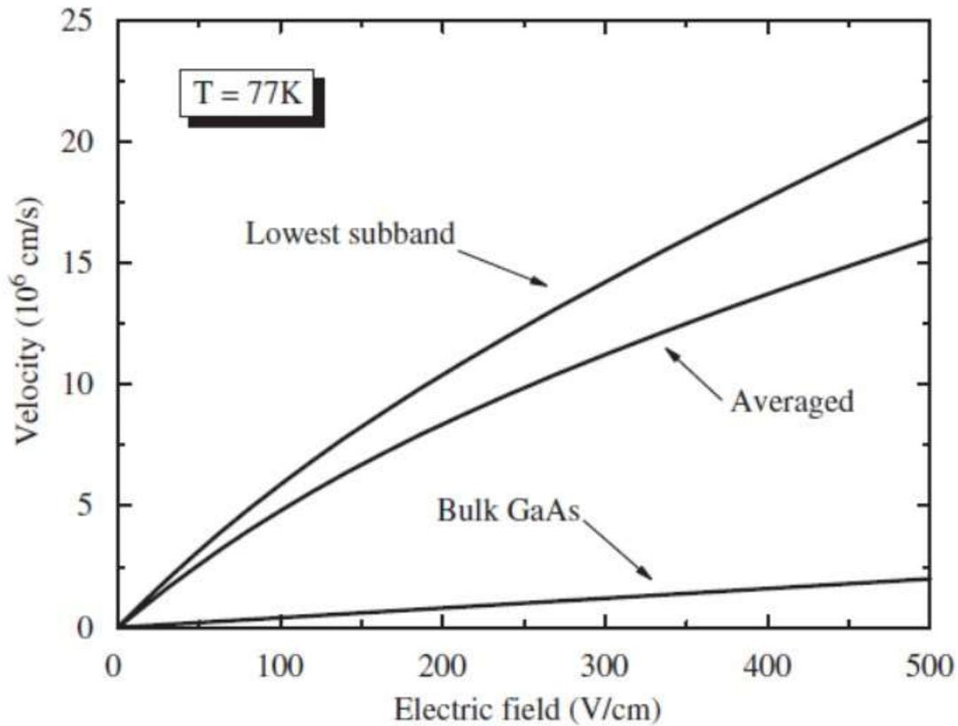
Electron drift velocity for parallel motion in AlGaAs–GaAs modulation-doped heterostructures
