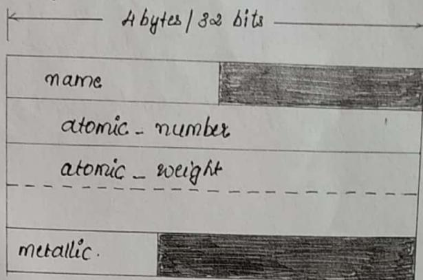
As the name field is only two characters long, it occupies two bytes in memory. Since atomic number is an integer and must be word aligned, there is a two-byte hole between the end of name and the beginning of atomic-number. Similarly in the case of Boolean variable (metallic).
