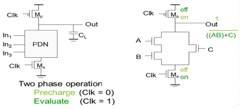
The logic is implemented using N type gates
