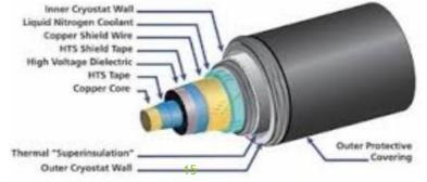
Example Superconductor cable design by Nexans
