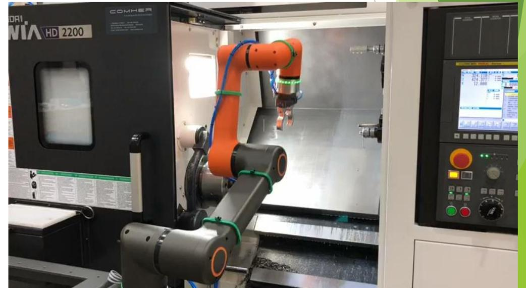
Machine Loading Robot
