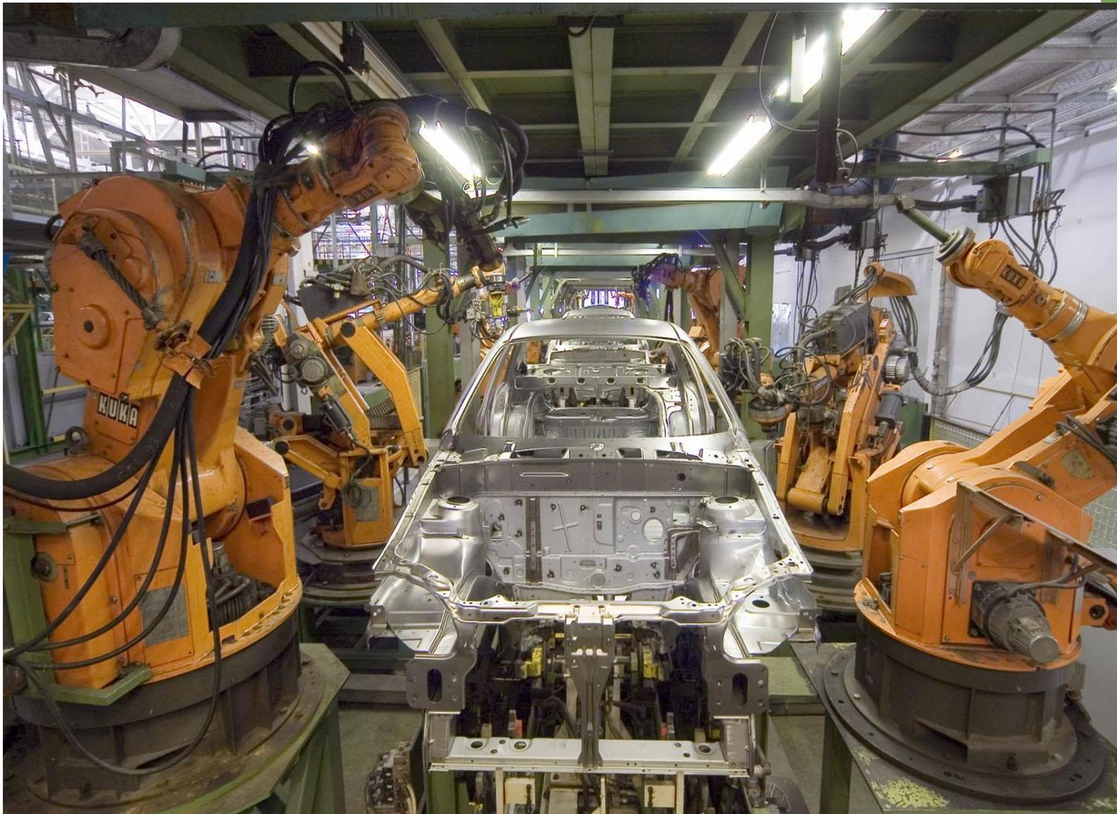
Industrial Robots being used for Automotive Manufacturing And Assembly
