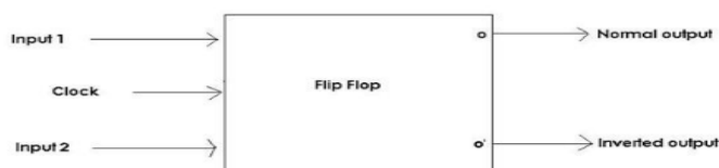
Fig 2. General block diagram of a Flip Flop
