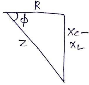
Where  $Z = R + j(X_C - X_L)$  is the impedance of series RLC circuit
