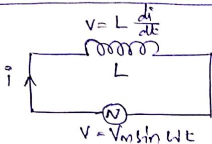
Consider an ac circuit consisting of pure inductance  $L$  Henry, to which an AC voltage  $V = V_m \sin \omega t$  is applied.
