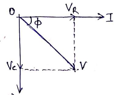
where  $Z = \sqrt{R^2 + X_C^2}$  is the impedance of series RC circuit.
