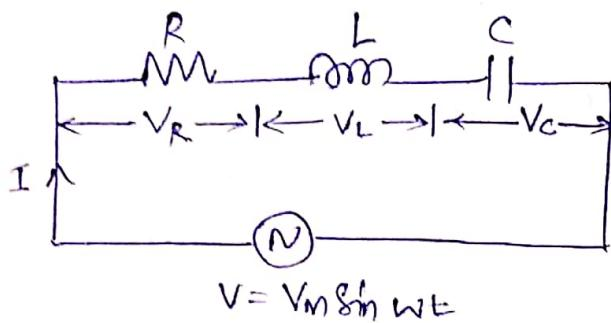
Consider an AC circuit consisting of a series combination of R, L and C elements. The behaviour of RLC circuits depend on the dominance of L and C elements.
