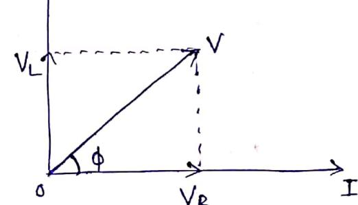
where  $Z = R + jX_L$  is called impedance of series RL circuit
