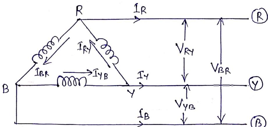
$V_{RY}$  is the voltage of terminal R w.r.t to Y. Similarly,  $V_{YB}$  is the voltage of Y w.r.t to B and  $V_{BR}$  is the voltage of B w.r.t to R.
