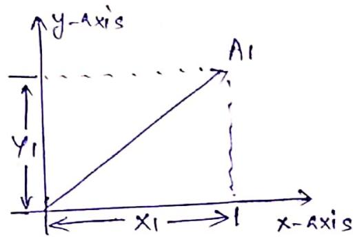
$x_1$  is called real component and  $y_1$  is called imaginary component. This is the rectangular form of phasor representation.
