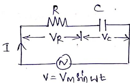
Consider an AC circuit consisting of a series combination of R and C.
