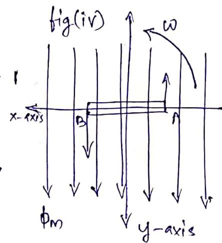
After  $270^\circ$  at instant 4, the conductor position falls similar to that at instant 2 as in figure(v). Point B moves towards right and point A towards left; both being llae to magnetic field. Hence flux cut is maximum and thus induced emf is maximum in the negative direction since at this instant, the conductor position is opposite to that at instant 2 even though similar.
