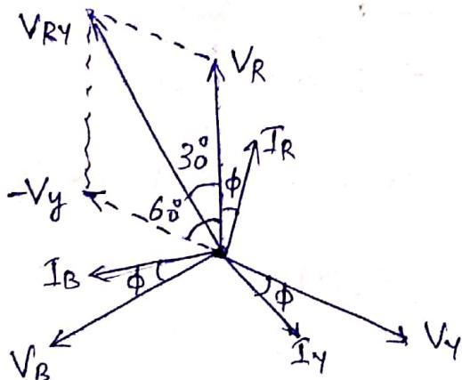
Line voltage  $V_{RY}$  is the vector difference of  $V_R$  and  $V_Y$ . (25)
