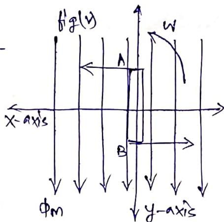
At any instant in between the induced emf ranges between zero and +ve or -ve maximum values.
