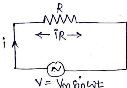
Consider an ac circuit consisting of pure resistance  $R \Omega$ , to which an ac voltage  $V = V_m \sin \omega t$  is applied.
