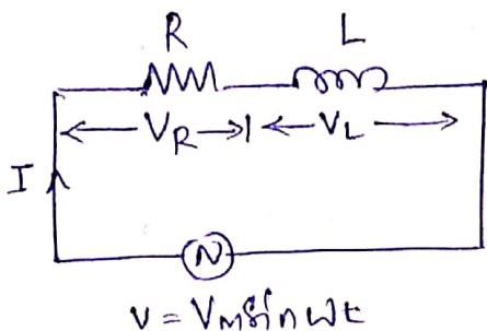
Consider an AC circuit consisting of a series combination of  $R$  and  $L$ .
