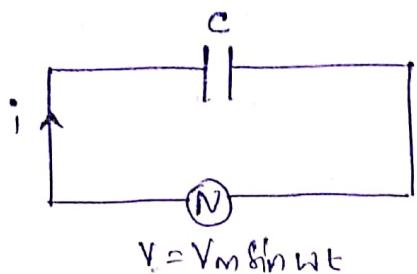
Consider an ac circuit consisting of pure capacitance  $C$  farad, to which an AC voltage  $V = V_m \sin \omega t$  is applied.
