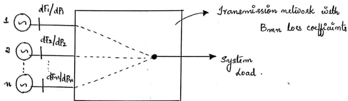
Let there are 'n' number of plants connected to a hypothetical load through a transmission network. The incremental cost of production at the  $n^{\text{th}}$  bus bar is  $dF_n/dP_n$ . Let there is an increase in power demand (load)  $\Delta P_D$ . Let this increase in demand is met by plant 'n' alone.
