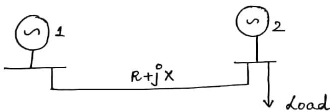
Here, 2 generators have equal incremental production cost. If generator 2 has a local load, according to equal production cost criteria, total load must be shared by the two. But common sense tells us that it is more economical to let Gen 2 supply most of the local load, because gen 1 has to supply in addition to the load, the transmission losses also. So here, equal incremental cost does not hold good, so we have to consider transmission losses also.
