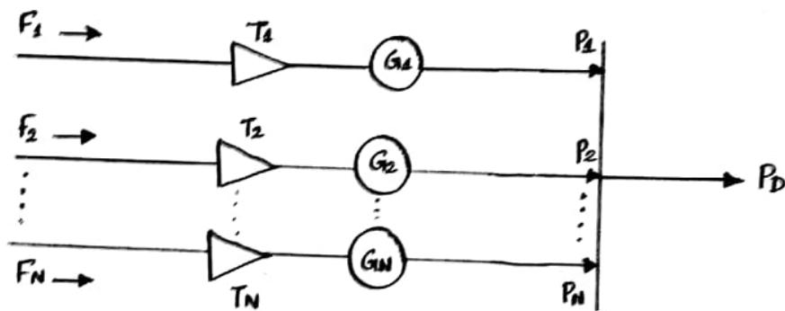
Our objective is to minimize the cost of production of power subjected to some constraint
