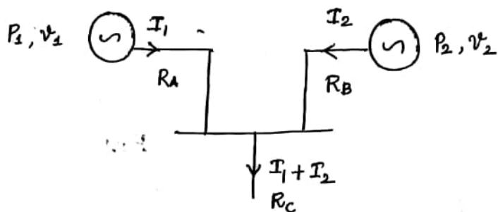
Let  $P_1, V_1, I_1, R_A, P_2, V_2, I_2, R_B, R_C$ , be the powers, voltage, current and Resistances of generator 1 and 2 respectively. From the single line diagram, the total transmission loss;  $P_L$  is:
