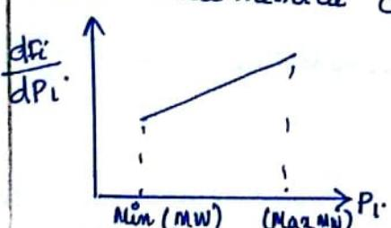
$$\therefore \text{Incremental Cost} = \frac{dF_i^o}{dP_i^o} \\ = a_i^o P_i^o + b_i^o$$
