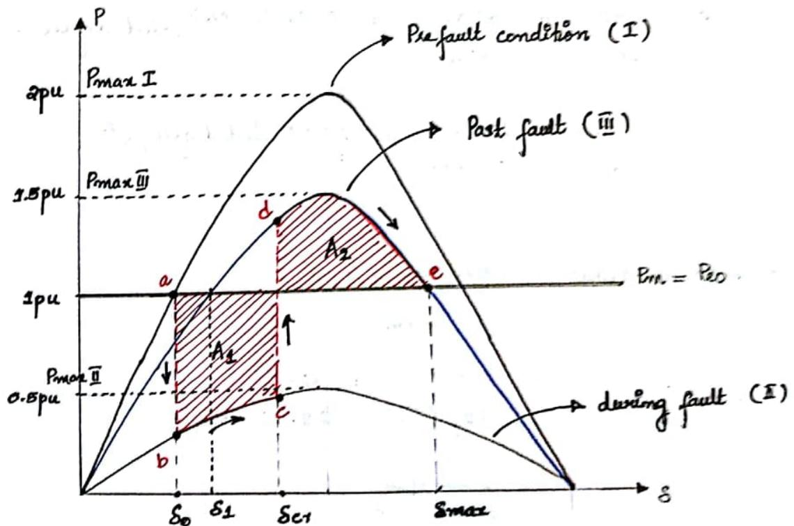
Let the s/m was operating under stable condition at point 'a'; where  $P_m = P_e = 1 \text{ p.u}$  in the I curve. Suddenly a fault occurs and the operating region falls from 'a' to 'b' in the II curve. Let at  $\delta_{cr}$ , the fault is cleared at point 'c' and operating region shifts to d in curve III.
