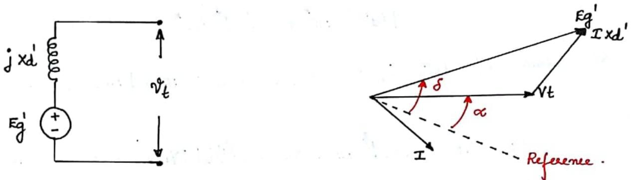
Let a single generator supplies power through a transmission line to a load or a large system at other end. Such a system can be represented by a 2 bus network as shown below.
