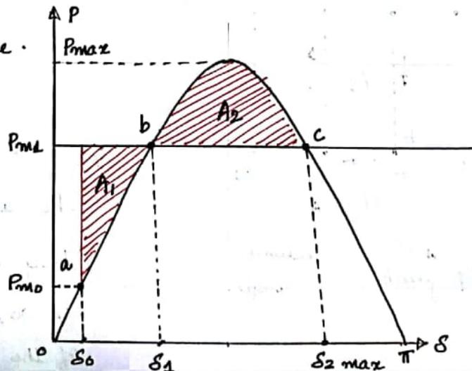
Any further increase in  $P_m$ , will reduce the area  $A_2$  and which violates the equal area criterion of transient stability.
