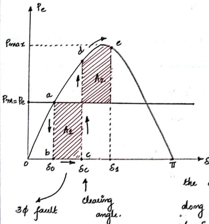
If a  $3\phi$  fault occurs at the point P of the outgoing radial line, the electrical output of the machine will reduce to zero. i.e.  $P_e = 0$ , hence the operating region shifts from 'a' to 'b'. Now  $P_a = P_m - P_e$  is +ve and the rotor accelerates and  $\delta$  increases. i.e., the accelerating area  $A_1$  starts increasing along bc. Let at time  $t = t_c$  corresponding to  $\delta_c$ , the fault is cleared, by the opening of the circuit breaker.
