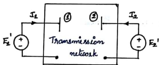
$E_1'$  = Transient internal voltage of generator at bus 1
