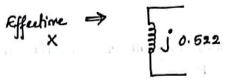
$$\begin{aligned} \therefore P_{max I} &= \frac{1.2 \times 1}{0.522} \\ &= \underline{\underline{2.29 \text{ p.u}}} \end{aligned}$$
