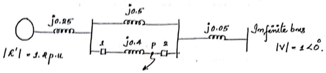
Find the critical angle for clearing the fault with simultaneous opening of the breakers 1 and 2. The reactance values of various components are indicated on the diagram. The generator is delivering 1.0 p.u power at the instant preceding the fault.
