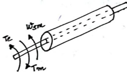
The rotor of a synchronous machine is subjected to two torques,  $T_e$  and  $T_m$ , which are acting in opposite directions.
