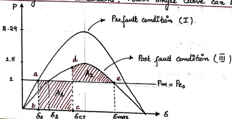
Let the system was operating under stable condition at point 'a'; where  $P_m = P_e = 1 \text{ p.u}$  in the I curve. Suddenly a fault occurs and the operating region shifts from 'a' to 'b'. The load angle continues to increase and let at  $\delta_{cr}$ , the fault is cleared and operating region shifts from 'c' to 'd' in curve III.
