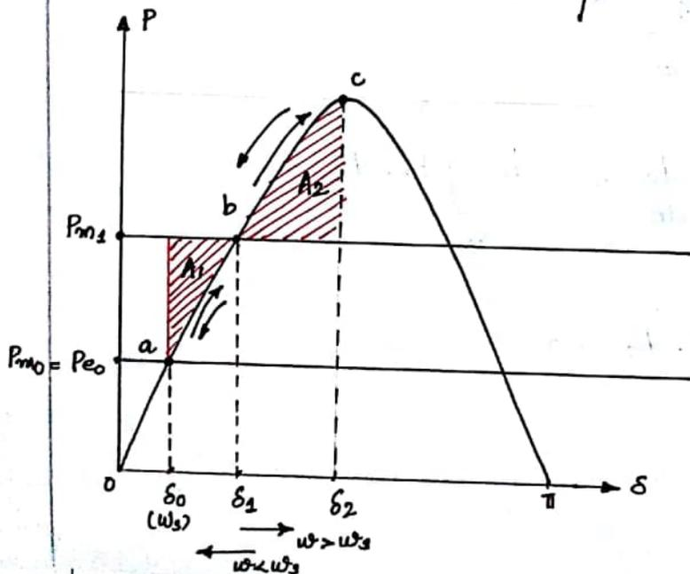
Let the mechanical input to the rotor is suddenly increased from  $P_{m0}$  to  $P_{m1}$ . Now the power  $P_a = P_{m1} - P_e$  is +ve and causes the rotor to accelerate and so does the rotor angle. As the angle increases from  $\delta_0$ , the
