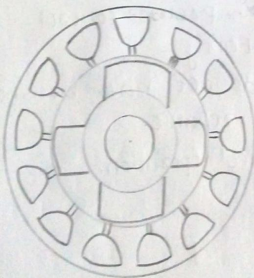
In an inner rotor design, the rotor is located in the centre of the motor.
