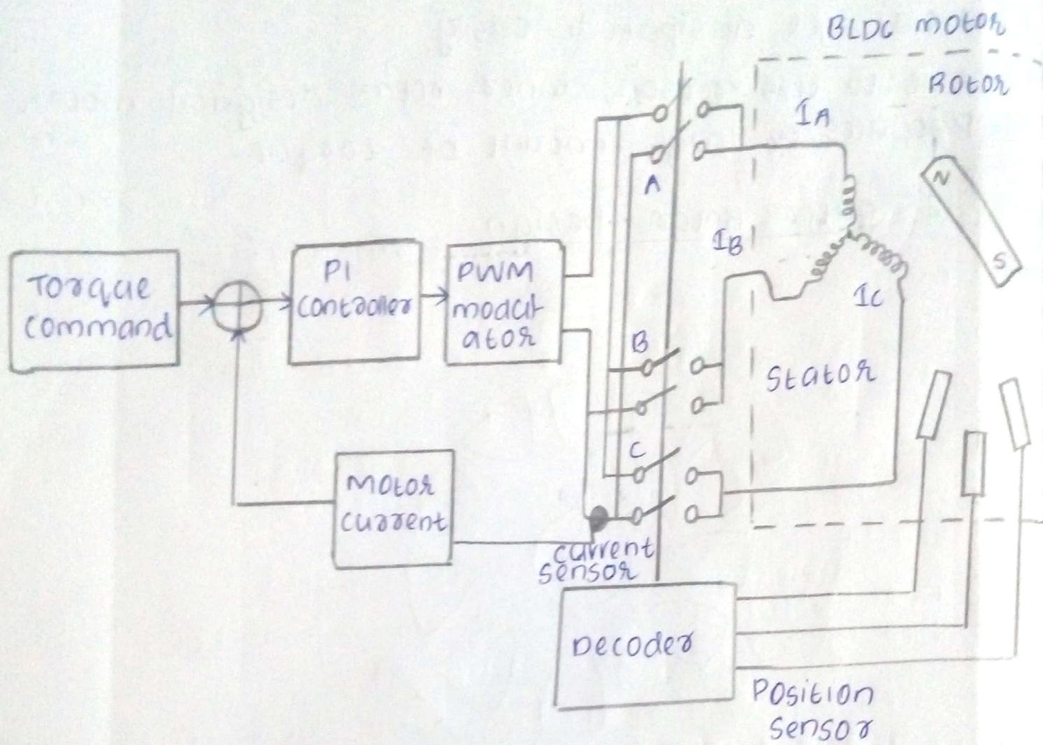
The figure shows the block diagram of trapezoidal type brushless DC motor.
