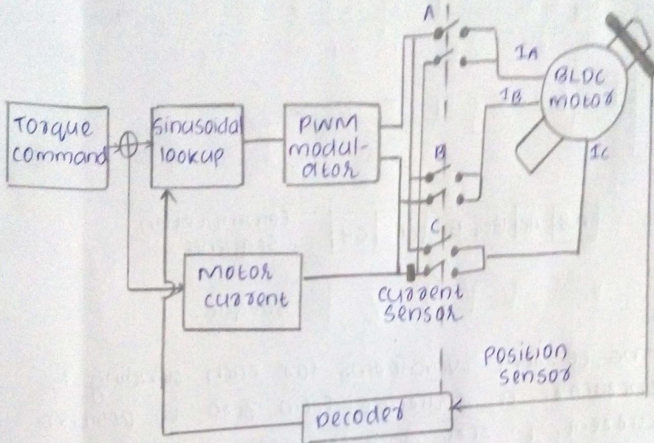
The figure shows the block diagram of sinusoidal type brushless DC motor.
