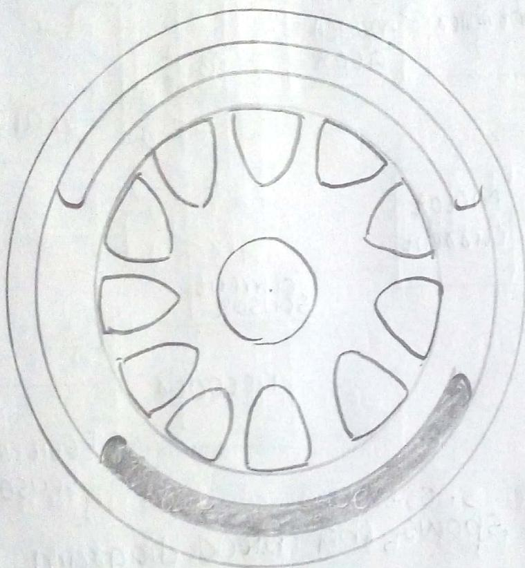
In outer rotor design, the rotor surrounds the winding, which is located in the core of the motor.
